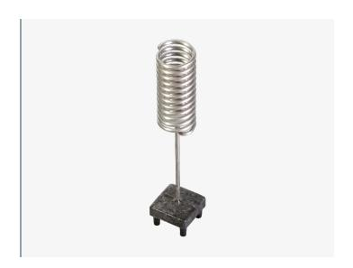
The 2.4 GHz Vertical Helical Antenna is a compact surface mount helical antenna designed for 2.4 GHz ISM frequency band applications such as Bluetooth® and ZigBee®. The 2.4 GHz Vertical Helical Antenna is made from 0.6 mm diameter nickel plated high-carbon steel for use in PCB-mount installations requiring a rugged, compact and omnidirectional embedded antenna. The connector-style base of the antenna ensures proper mounting for uniform performance in high-volume manufacturing.
